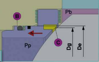
Double piston effect case A: the pressure in the pipeline (Pp) pushes the seat towards the ball.
