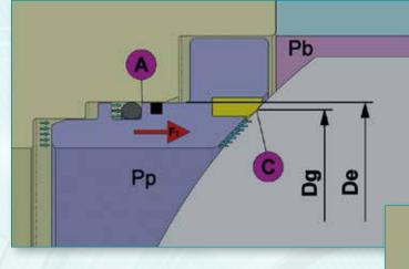
Single piston effect seat (Self-Relieving seat) case B: the pressure in the body cavity (Pb) pushes back the seat; the fluid can pass and relieve. Single piston effect seat (Self-Relieving seat) case A: the pressure in the pipeline (Pp) pushes the seat towards the ball.
