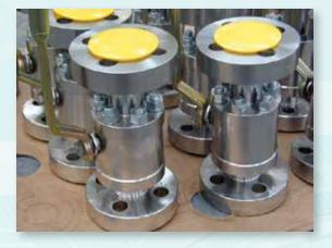
Floating ball valves have a simple structure: the ball is supported by the seats but can float inside the valve body.
