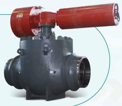
Top Entry ball valve design is characterized by one piece body construction with top access to all internal components. Top Entry Ball Valves are the preferable solution when it is required to perform in line maintenance, and when the reduction of possible leakage path is mandatory. The body could be manufactured from forged billet or high quality castings. Same options and features of side entry Trunnion ball valve are available also for top entry ball valves.
