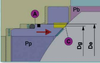
Double piston effect case B: the seat design permits the pressure in the body cavity (Pb) to push the same seat towards the ball.
